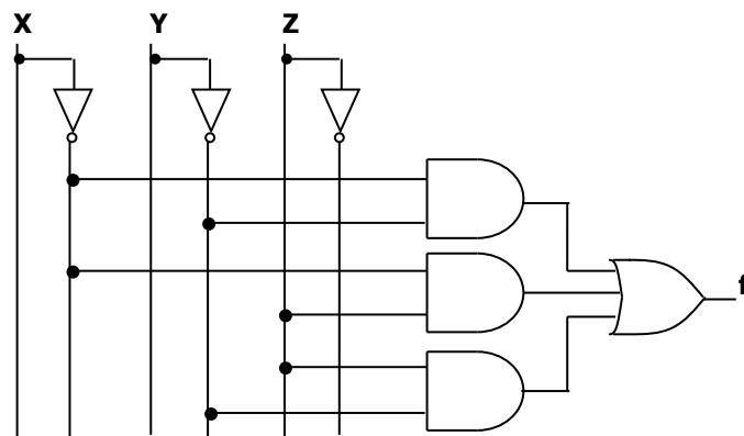
✓  $F = (Z + \bar{Y})(\bar{Z} + X)(\bar{Y} + X) = (Z + \bar{Y})(\bar{Z} + X)$  (Consensus Theorem)
